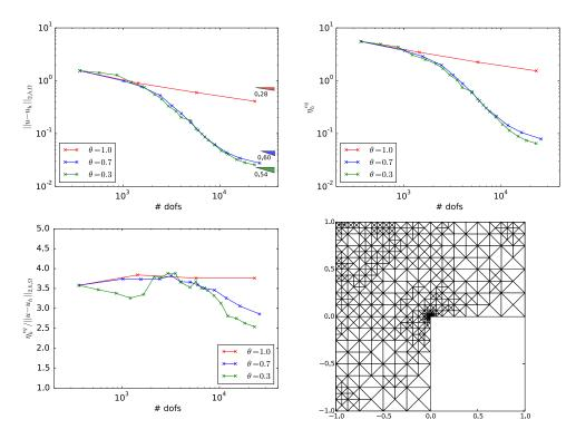
FIG. 8.3. Error, estimator, effectivity index, and adaptively generated mesh (k = 4).
