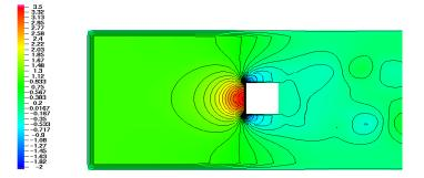
Figure 13: Problem Q2 (Re=100): The midplane pressure contours around a square cylinder. The solution shown was computed with  $h_{\text{max}} = 1/256$  and  $h_{\text{min}} = 1/1024$  at t = 16.
