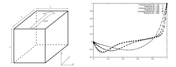
Figure 6: Left: The 3D driven cavity problem setup; Right: The centerline ((0.5, 0.5, z),  $0 \le z \le 1$ ) *u*-velocities compared to reference data from [33]
