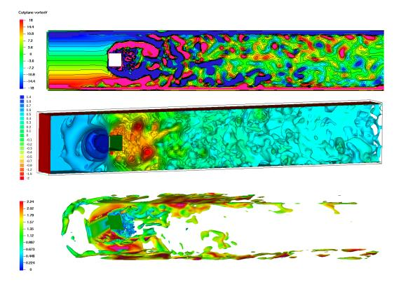
Figure 17: Channel flow around a square cylinder at Re=10000: Spanwise vorticity for the midplane y = 0.205. Pressure isosurfaces and vorticity isosurface  $|\mathbf{w}| = 100$  colored by the absolute velocity. The plots illustrate solution computed with  $h_{\text{max}} = 1/256$  and  $h_{\text{min}} = 1/1024$  at t = 8.
