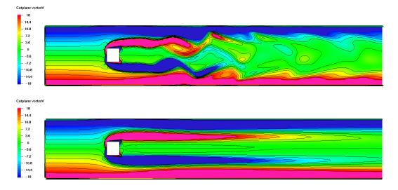
Figure 12: Problem Q2 (Re=100): Spanwise vorticity at time t=16 for the midplane y = 0.205. The top plot shows the development of vortex street for solution by BDF2 with FD advective terms; the bottom plot shows an over-diffusive solution computed by BDF2 with semi-Lagrangian method (linear interpolation). Both solutions were computed with  $h_{\text{max}} = 1/256$  and  $h_{\text{min}} = 1/1024$  at t = 16.
