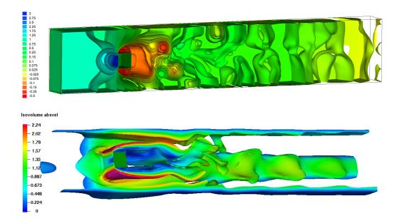
Figure 15: Problem Q2 (Re=100): Pressure isosurfaces and vorticity isosurface  $|\mathbf{w}| = 20$  colored by the absolute velocity. The plots illustrate solution computed with  $h_{\text{max}} = 1/256$  and  $h_{\text{min}} = 1/1024$  at t = 16.
