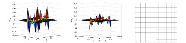
Figure 2: The velocity error is dominated by the div-free modes occurring on the coarse-to-fine grids interface. The left figure shows the *u*-component of the error, the middle figure shows the *v*-component, and the right figure shows the grid for h = 1/8.
