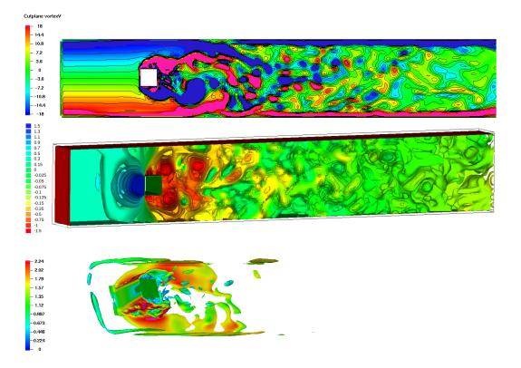
Figure 16: Channel flow around a square cylinder at Re=1000: Spanwise vorticity for the midplane y = 0.205. Pressure isosurfaces and vorticity isosurface  $|\mathbf{w}| = 100$  colored by the absolute velocity. The plots illustrate solution computed with  $h_{\text{max}} = 1/256$  and  $h_{\text{min}} = 1/1024$  at t = 8.
