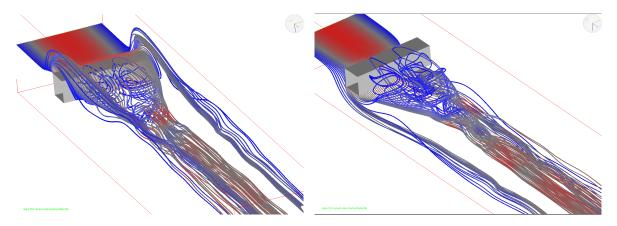
Figure 14: Problem Q2: Streamlines of the developed flow around a square cylinder for Re=100. The streamlines are selected for two fluid layers entering the domain slightly above and below x = 0.21.
