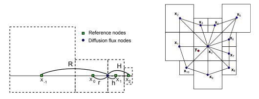
Figure 5: Left: Reference points for the diffusion flux approximation; Right:  $u_h(\mathbf{y})$  is defined by a linear interpolation based on the fan triangulation with the center in  $\mathbf{x}_V$ , i.e. interpolation of  $u_h(\mathbf{x}_V)$ ,  $u_h(\mathbf{x}_1)$ ,  $u_h(\mathbf{x}_{10})$  in this example.
