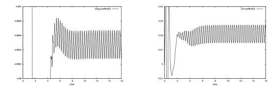
Figure 11: The evolution of drag (left) and lift (right) coefficients for the flow around a square cylinder with Re = 100 (problem Q2) computed with  $h_{max} = 1/32$ ,  $h_{min} = 1/1024$ .
