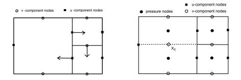
Figure 3: Left: A single local div-free mode, which is subgrid for the coarse grid cell. Right: Introducing additional pressure d.o.f. for the coarse cell next to fine cells. This yields a stronger discrete div-free condition and precludes the occurrence of subgrid div-free modes such as shown in the left figure.
