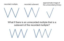
Figure 1: Using a recorded multiple to find an approximate image of an unrecorded primary of the multiple: illustrate the need to remove unrecorded multiples. A solid line  $(\_\_)$  is a recorded event, and a dashed line  $(\_--)$  connotes an unrecorded event.
