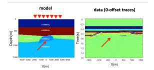
Figure 4: The model and zero offset traces of data. The base salt is almost invisible because the primary generated by the base salt is negatively interfering with an internal multiple.
