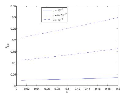
Figure 3.3: The values of  $P_{bot}$  as computed from different values of  $\mu$  and s, using the function  $\zeta_{\tau}(s)$ . We see  $0.0025 \leq P_{bot} \leq 0.3$ .  $P_{bot}$  increases with increasing s and  $\mu$ .
