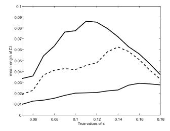
Figure 4.9: The mean length of CI of estimation for  $\hat{s}$  is plotted as a function of s for fixed  $\mu$ , based on an observation of a single population ( $\mathcal{N}=1$ ). The solid lines display the curves for two extreme range values for  $\mu=2\times10^{-8}$  (bottom solid line) and for  $\mu=10^{-6}$  (top solid line). The dotted line displays the mean length of CI for a mid-range values of  $\mu=5\times10^{-7}$ .
