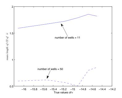
Figure 4.17: This figure displays the mean length of the confidence intervals for true values of  $\nu$ , for a fixed s=0.10, and for different  $\mathcal{N}=11,50$ . The mean length of the confidence intervals decreases as the number of wells  $\mathcal{N}$  increases.
