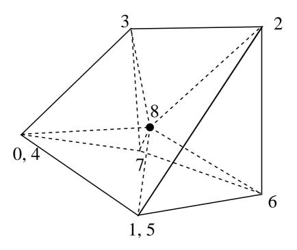
Figure 3.12: Partition of a prism into three pyramids and two tetrahedrons
