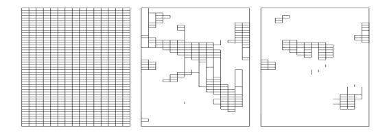
Figure 2.4: Graphs of the diagonal blocks of the matrices  $A_0$  (left),  $A_1$  (center) and  $A_2$  (right) for a "horizontal" mesh plane
