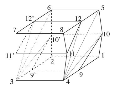
Figure 3.20: An example of splitting the hexahedron into triangular prisms
