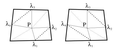
Figure 3.26: Connections p-p and  $p-\lambda$  for the "Splitting One" (left) and "Splitting Two" (right)
