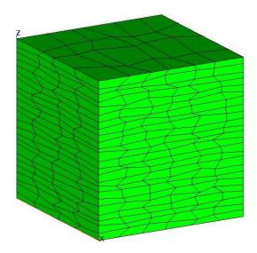
Figure 3.30: Example of a hexahedral mesh  $(4 \times 6 \times 24)$
