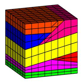
Figure 3.21: An example of a mesh with pinchouts
