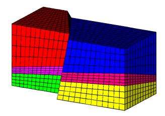
Figure 3.2: Distorted hexahedral mesh with a fault
