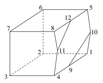
Figure 3.17: An example of a fault hexahedral cell E
