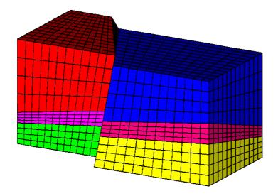
Figure 3.22: An example of a mesh with a fault
