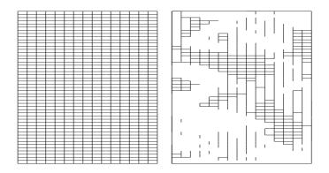
Figure 2.1: Graphs of the diagonal blocks of the matrices A (left) and  $A_1$  (right) for a "horizontal" mesh plane
