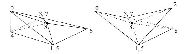
Figure 3.15: Subcells  $e_1$  (left) and  $e_2$  (right) for a H2 element
