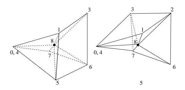
Figure 3.11: Subcells  $e_1$  (left) and  $e_2$  (right) for a H1 element
