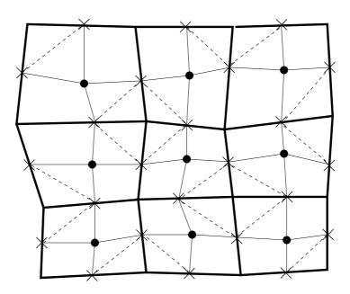
Figure 3.27: p - p and  $p - \lambda$  connections for the matrix  $A_{p,\lambda}$
