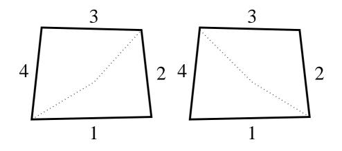
Figure 3.25: "Splitting One" (left) and "Splitting Two" (right) of a quadrilateral cell
