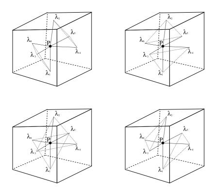
Figure 3.29: Connections p-p and  $p-\lambda$  for different splittings of a hexahedral cell
