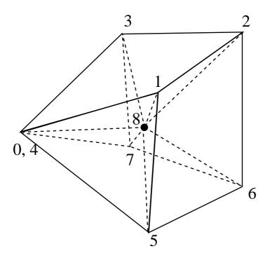
Figure 3.10: Partition of a H1 element into four pyramids and two tetrahedrons
