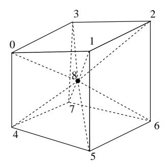
Figure 3.8: Partition of a distorted hexahedron into six pyramids
