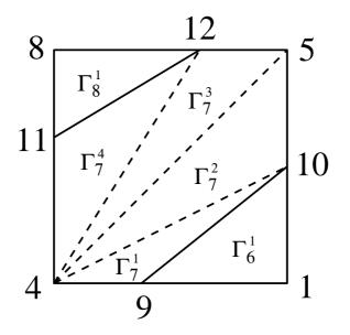
Figure 3.19: An example of the triangulation of a fault face
