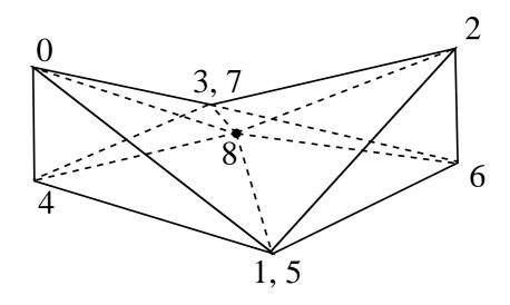
Figure 3.14: Partition of an element H2 into two pyramids and four tetrahedrons
