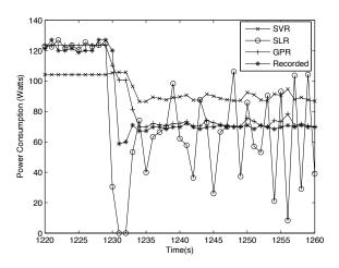
Figure 3: A part (80 seconds) of cross-validation comparison results when a NVidia CUDA SDK sample "OceanFFT" ran on NVidia GeForce 8800 GT.
