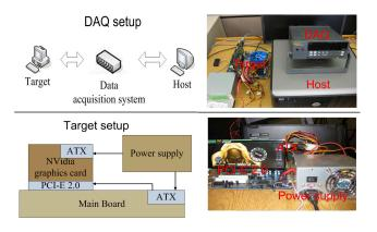
Figure 1: Data acquisition setup used in this work. Note that the graphics card had two power supplies (ATX and PCI-E 2.0). DAQ is a FLUKE Hydra logger 2625A power acquisition system, and the target computer is equipped with the chosen NVidia GeForce 8800 GT graphics card (200 Watt power specification), AMD Athlon 64x2 3.0GHz Dual-Core Processor, 2GB memory, and Corsair TX750W power supply.
