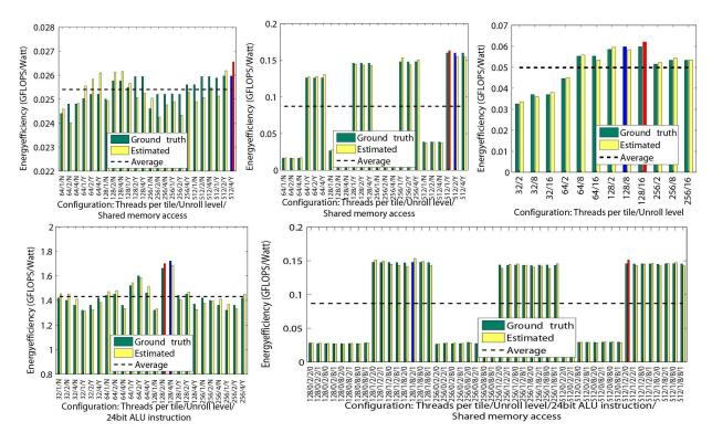
Figure 4: The estimated and ground-truth energy-efficiencies for all the generated candidates of the selected benchmarks (from top-left to bottom-right): "particles", "matrixMul", "scalarProd", "MersenneTwister", and "fastWalshTransform". The blue bars indicate the candidates of maximal ground truth energy-efficiencies while the red bars indicate the candidates of maximal estimated energy-efficiencies.
