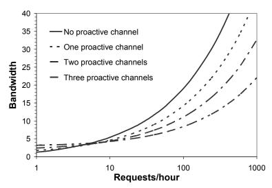
Fig. 5. Bandwidth requirements of the stream tapping protocol for a two-hour video with and without proactive streams.
