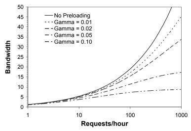
Fig. 4. Bandwidth requirements of the stream tapping protocol for a two-hour video when various fractions  $\gamma$  of the video are preloaded.
