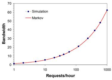
Fig. 2. Bandwidth requirements of the stream tapping protocol for a two-hour video.
