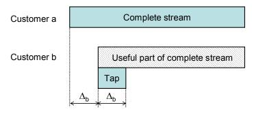
Figure 1: How stream tapping works
