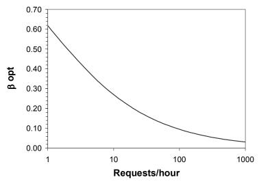
Fig. 3. Fraction of a two-hour video that the client must be able to store in order to achieve the best performance at different request arrival rates.
