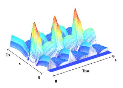
Figure 7: Shear stress on the *moving* lower wall.
