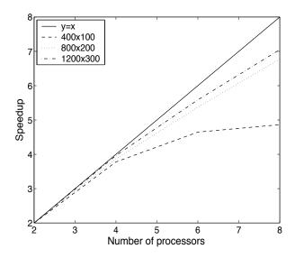
Figure 12: Parallel speed-up for the parallel Navier-Stokes code.
