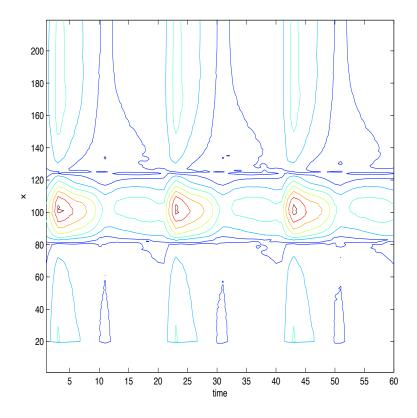
Figure 8: Contour plot of the Shear stress on the moving lower wall.
