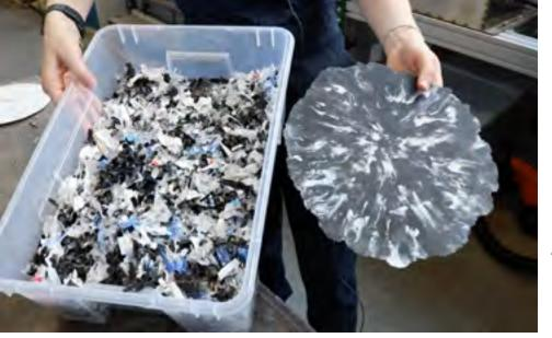
**ABOVE:** PLASTIC IS CLEANED AND SHREDDED BEFORE BEING FORMED INTO A SHEET OR BLOCK
